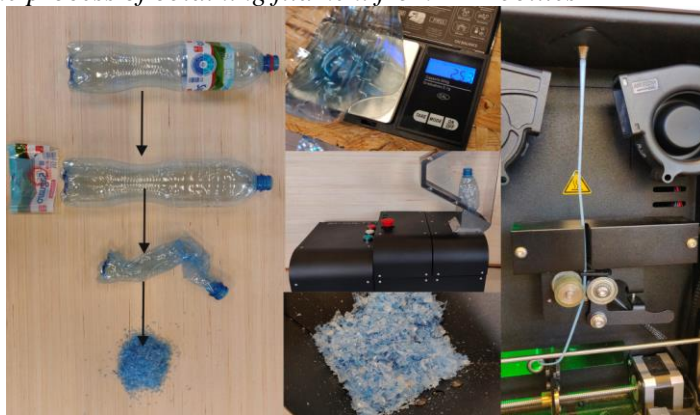
Figure 2. The process of obtaining filament from PET bottles
